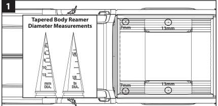
Using the molded-in dimples in the truck bed as a guide, carefully cut two front 7mm (0.275") holes and two rear 13mm (0.5") holes in the bed with a tapered body reamer to allow clearance for the screw bosses on the roll bar and mounts (note the hole diameter measurements on the body reamer).
