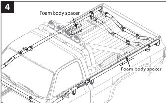
Remove the existing foam body spacers (2) from the flat surfaces on the body cage (underside of body) as shown, and then peel the backing from the new foam body spacers and attach them in the same locations. Reinstall the clipless latch.
