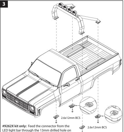
the left side (driver side). Secure the roll bar to the truck body as shown using the included roll
