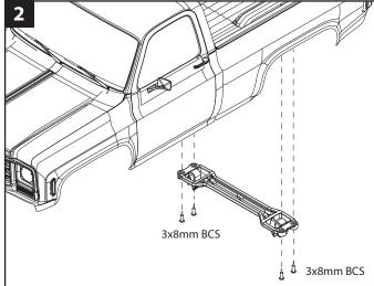
Remove the rear clipless latch by removing the 3x8 BCS (4).
